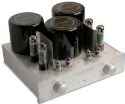
The stainless steel panels between the mains power transformer and output valves reduce the transformers' running temperature and shield the output valves improving over all amplifier efficiency and sound quality.
