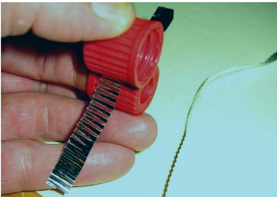
Corrugate the alu foil between the two screw caps as seen here. This takes some practice and people have produced all sorts of nice machinery for this, but we only have to corrugate 10 cm of foil, so this can all be done by hand as seen here.
